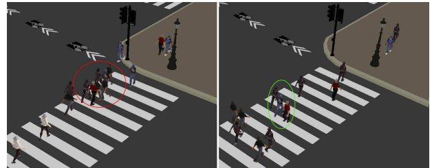
Fig. 10 - Left, collision avoidance is deactivated. Right, collision avoidance is activated.
