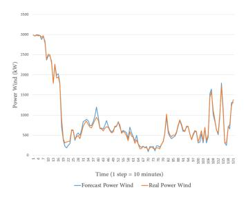
Fig. 4. Graph of the forecast provided by AMOEBA and the real wind power of a wind turbine of the wind farm in France during more than 20 hours. The historical data set for learning and resolution steps is made with data of the force of the wind at the basket of the wind turbine and the corresponding production from 2015.
