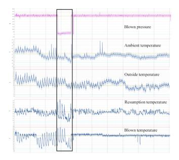
Fig. 5. The period is between october 12 and december 21 2014. The pressure is between 0 and 450 Pa. The ambient temperature is between 19 and 28 C. The outside temperature is between 1 and 31 C. The discard temperature is between 9 and 33 C. The blown temperature is between 10 and 28 C.
